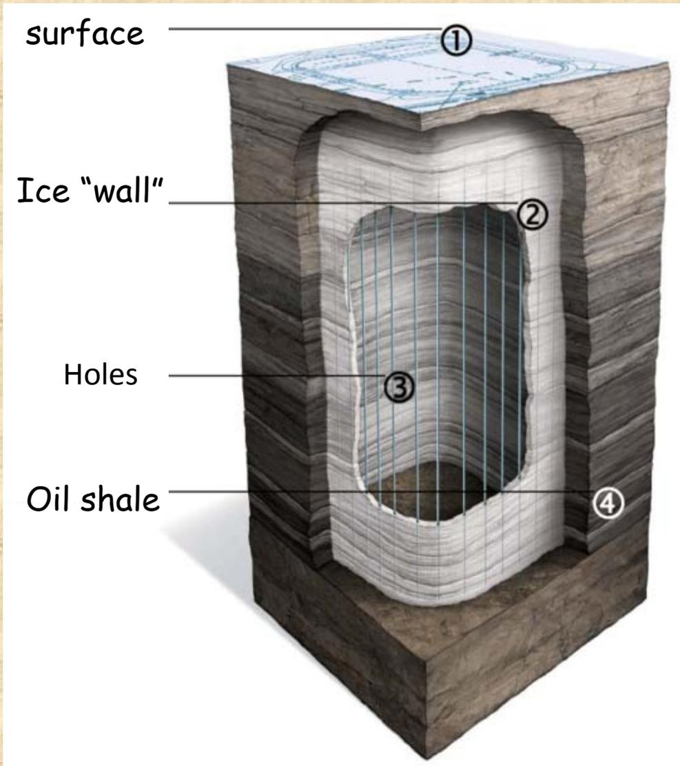
Before heating and exploitation groundwater is eliminated by creating an "ice wall"
