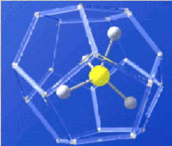
Crystalline water-based solids in which small non polar molecules (typically gases: methane,  $\text{CO}_2$ ...) are trapped inside “cages” of hydrogen bonded water molecules
