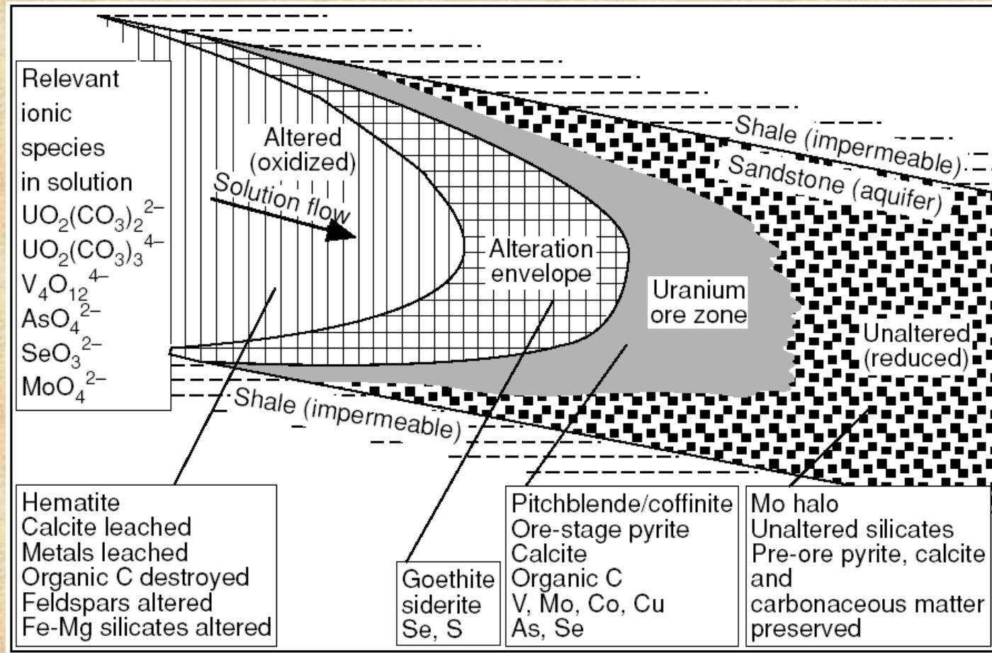
**Typical redox front**, which behaves as a uranium trap, in sandstone (“roll-front uranium deposit”)
